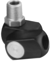
Dynaswivel® Swivels 360° at two locations which allows an air hose to drop straight to the floor, no matter how the tool is held. • 94300 1/4" NPT
