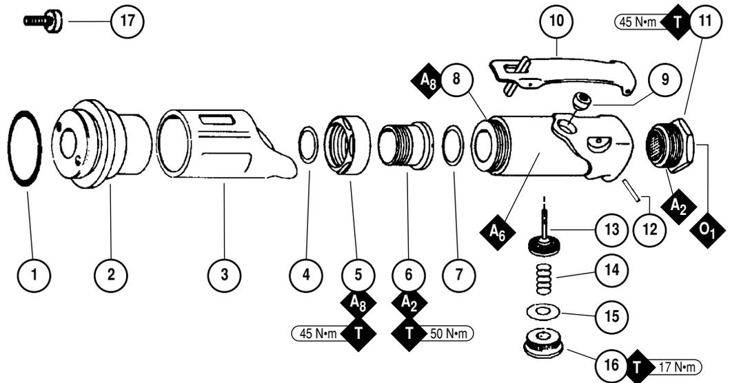
**Note:** On Models 14302, 14303, and 14306 the 07167 Throttle Valve Assembly can be mounted on either side of the tool for right or left hand comfort.
