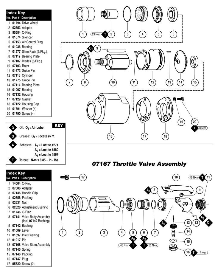
Note: On Models 14302, 14303, and 14306 the 07167 Throttle Valve Assembly can be mounted on either side of the tool for right or left hand comfort.
