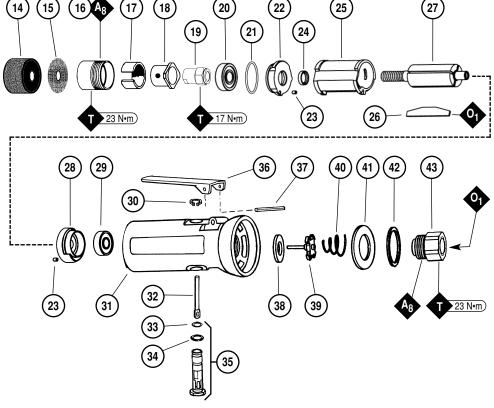
Note: 50971 Lock Ring Wrench is available for removal/installation of 04087 Lock Ring. See inside for Important Operating, Maintenance and Safety Instructions before operating tool.
