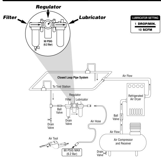
Ideally the air supply should be free from moisture. Incorporating a refrigerated air dryer after the compressor and drain valves at each tool station (as shown) further reduces moisture from condensation in the air supply.  Dynabrade Air Power Tools are designed to operate at 90 PSIG (6.2 Bar/620 kPa) maximum air pressure at the tool inlet, when the tool is running. Use recommended regulator to control air pressure.
