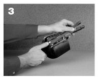
Depress idler arm lever and pull belt toward the contact wheel.
