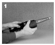
With your thumb, pull and slide guard open in a clockwise direction.
