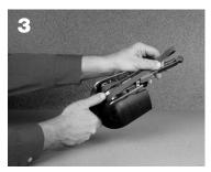
Depress idler arm lever and pull belt toward the contact wheel.
