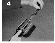
Slip belt over contact wheel. Release idler arm lever. Operate on the contact wheel or on the return side of the belt.
